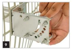
U-Bolts & toothed saddle should be positioned as shown for the best grab on the mast. Position feedhorn so bolts & connector pass through reflector. Place L-Bracket over bolts and connectors as shown.
