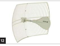
Completed Antenna NOTE: The antenna has a very narrow radiation beam. Antenna will only work within the narrow signal cone.
